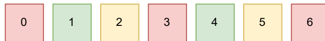
Figure 4: User Defined Scheduling / Ordered / Block Size of One. Colors refer to Threads
